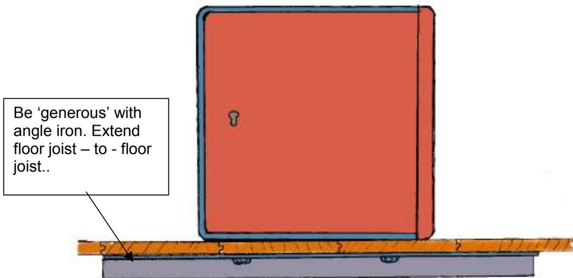
If you must leave the nuts under the floor, burr the thread so that they cannot be removed or weld the nuts to the plate or angle iron as extra security.
